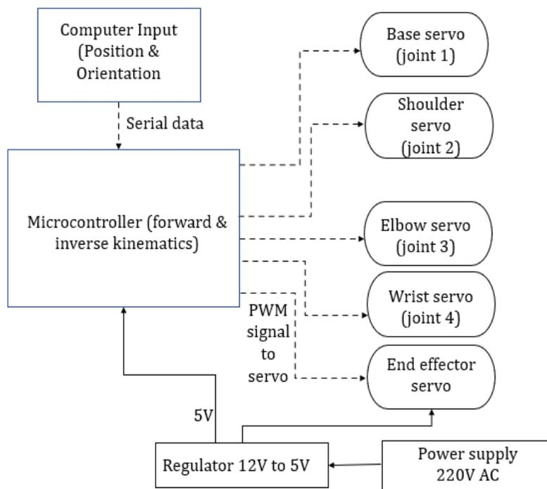
**Figure 8.** Experimental Setup for Kinematic Models Validation
