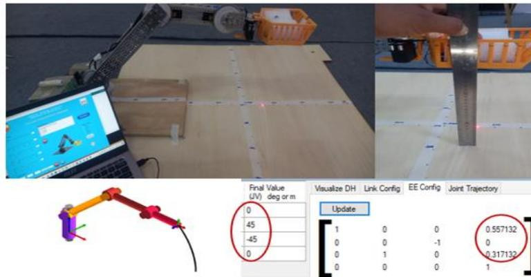
**Figure 9.** Experimental Result for Point1 (0, 45, -45, 0)
