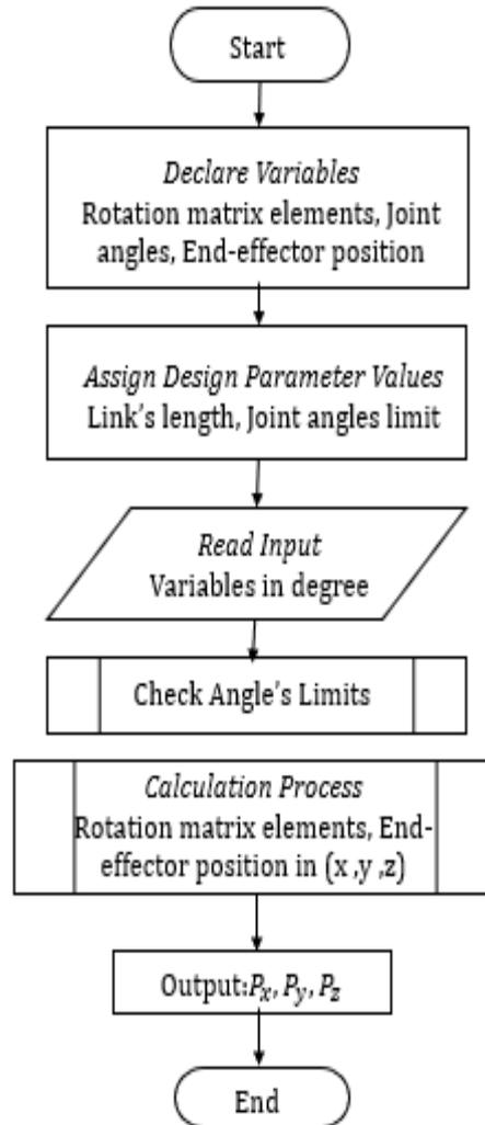
**Figure 6.** Flowchart of Forward Kinematics Modeling Algorithm
