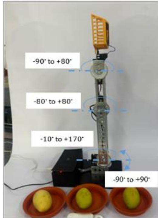
**Figure3.** Orientation Angle of Four Links Articulated Robot
