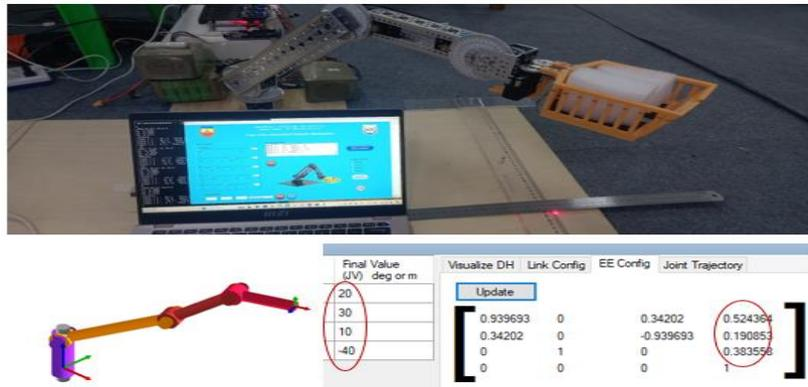
**Figure12.** Experimental Result for Position 4 (20,30, 10, -40)
