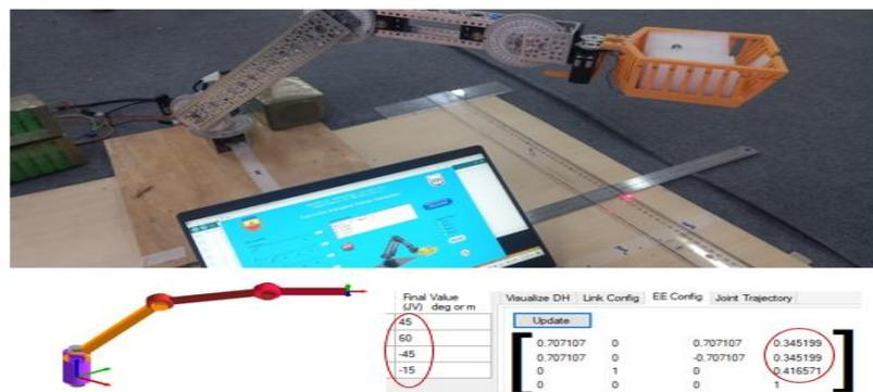
**Figure10.** Experimental Result for Position 2 (45,60, -45, -15)
