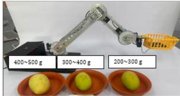
**Figure2.** Four Links Articulated Robot for Sorting System
