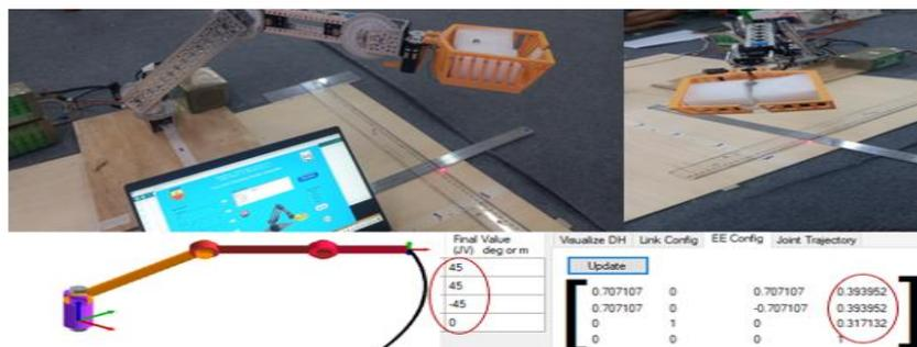
**Figure11.** Experimental Result for Position 3 (45,45, -45, 0)
