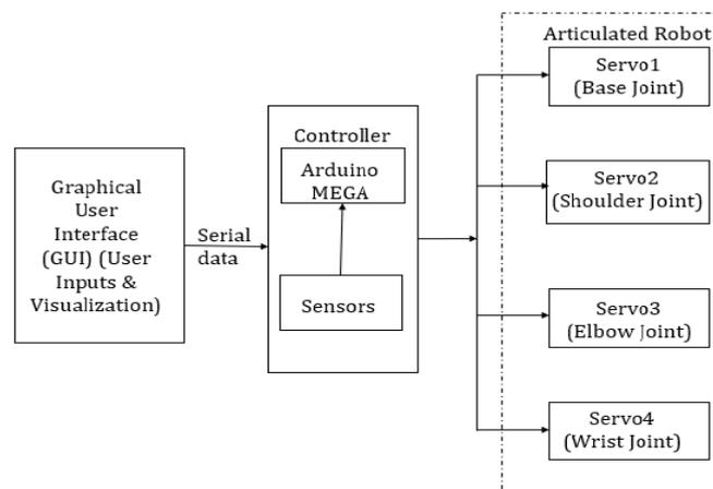
**Figure 1.** System Block Diagram of Four Links Articulated Robot
