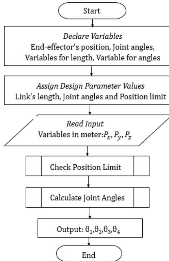
Figure.7. Flowchart of Inverse Kinematics Modeling Algorithm
