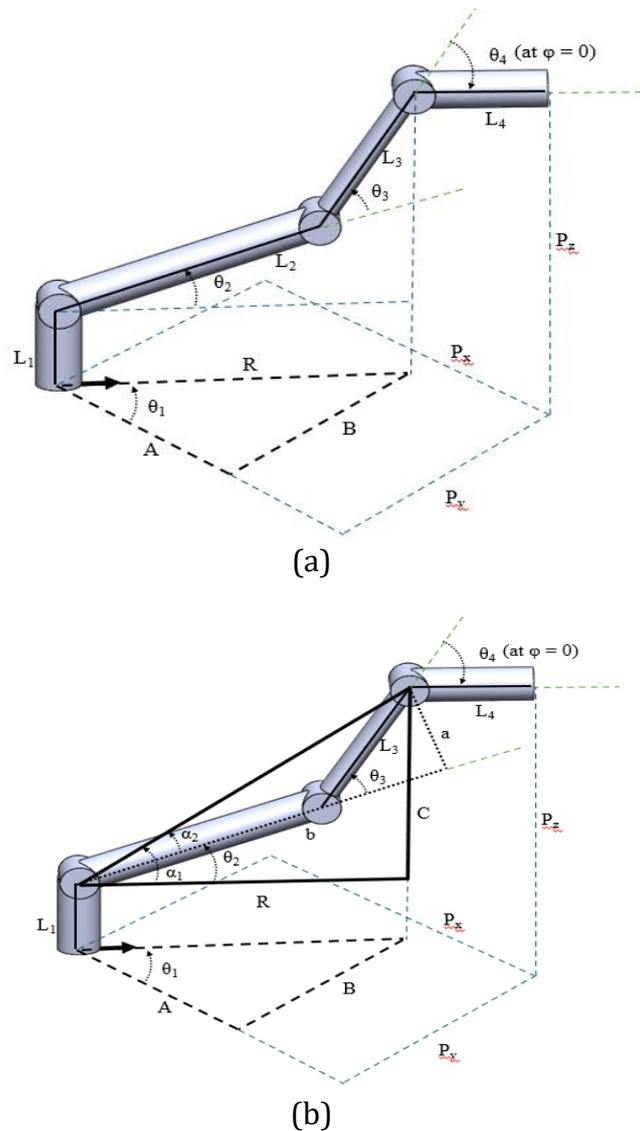
**Figure 5. (a,b) Elbow Down Condition for Four Links Articulated Robot**
