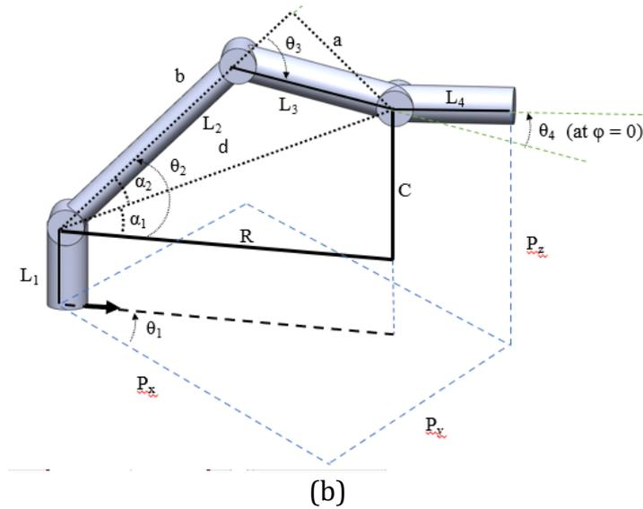
Figure 4. (a,b) Elbow Up Condition for Four Links Articulated Robot
