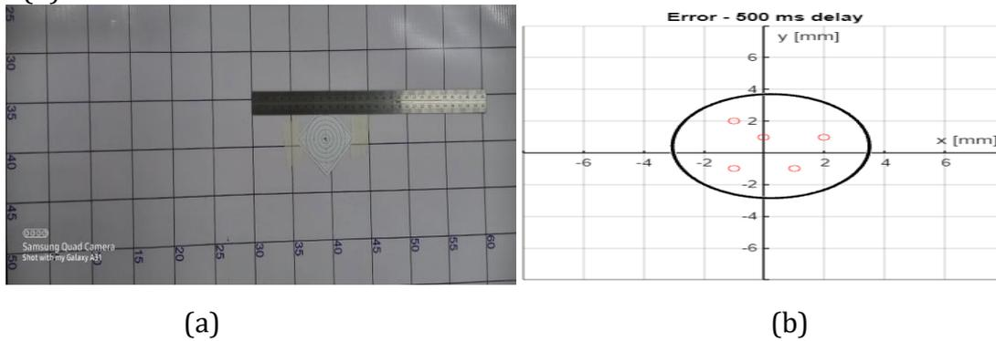
**Figure 16.(a,b)** Experimental Result for Position 3 (45, 45, -45, 0)
